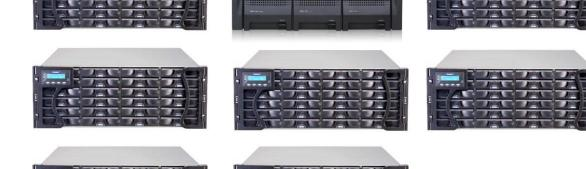
dual redundant 8 Gb FC controllers with 4 GB cache per controller and 3, 4, or 8 TB SATA or SAS hard drives configured with RAID 6
